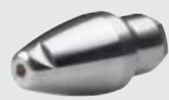
z0000116 Falch pointspeed 5 one, 500 bar, 20°, 020, 90° C, 1/4" ig, V2a
